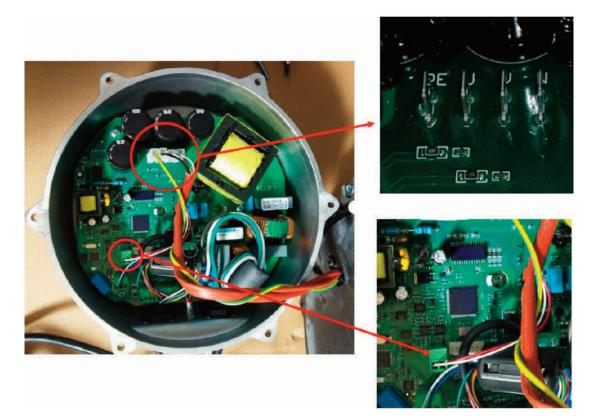
Disconnect the fastons on the motor phase electronics and probe
