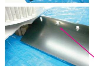
TOP PART OF THE BLADE FIXED WITH THE SELF-LOCKING NUTS
