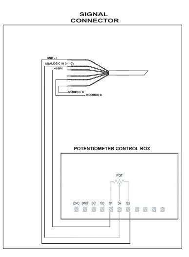
NB: It is necessary pull the A and B wires down to the control box for the Modbus connection, used for maintenance and diagnostic actions.
