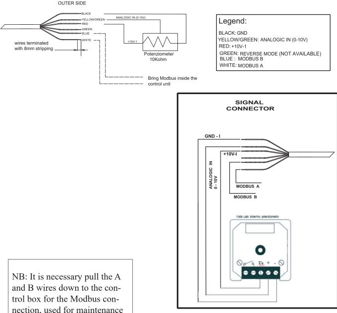
nection, used for maintenance and diagnostic actions.
