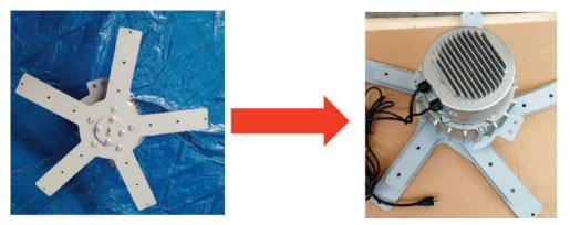
To assemble the bracket, you need to rotate the motor, resting it on the starwheel. Position the bracket over the motor so as to centre the holes on the fall protection plate.
