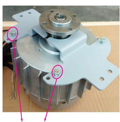
Remove the screws fixing the fall protection plate to the motor
