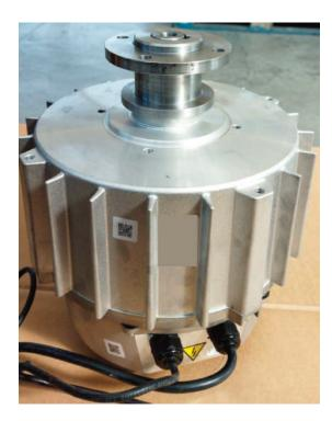
Insert the hub on the shaft in the direction indicated in the figures. The narrower cylindrical part must be touching the motor.
