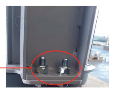
After having set the inverter motor on the ground, remove the bracket fixing screws.
