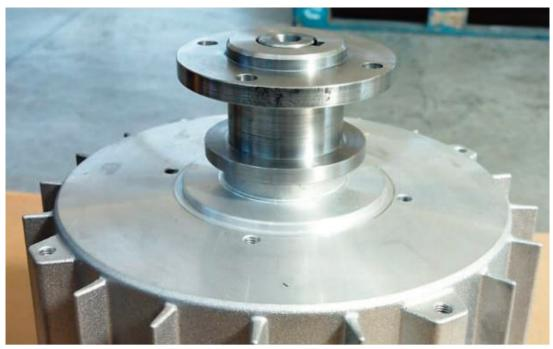
Slide off the fall protection plates and remove the hub from the shaft
