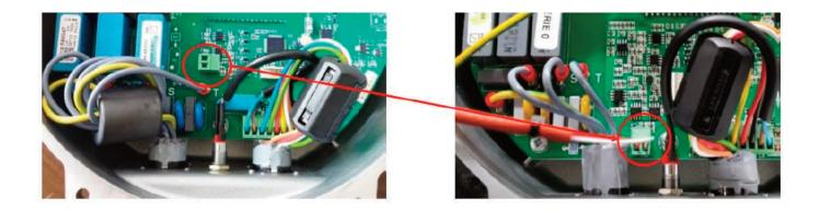
Insert the motor temperature sensor green connector, with White/Red wires, in the corresponding connector on the electronics (positioned as shown in the figure).
