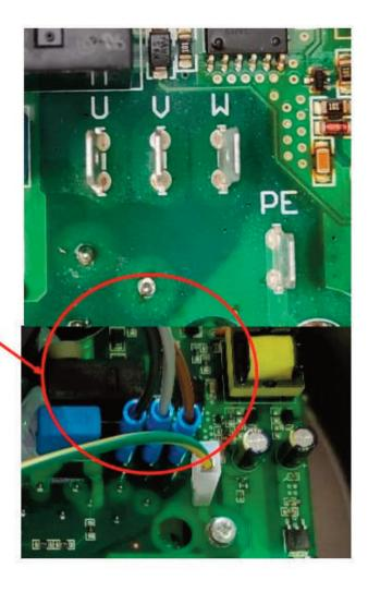
Insert the faston connectors on the motor phase electronics according to the following diagram:
